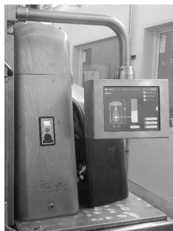
Shown here is the screen attached to each robotic milking machine showing the various data being collected about the cow currently in the machine, including the amount of milk being collected. The machine is fully automated, but can also be manually operated.
